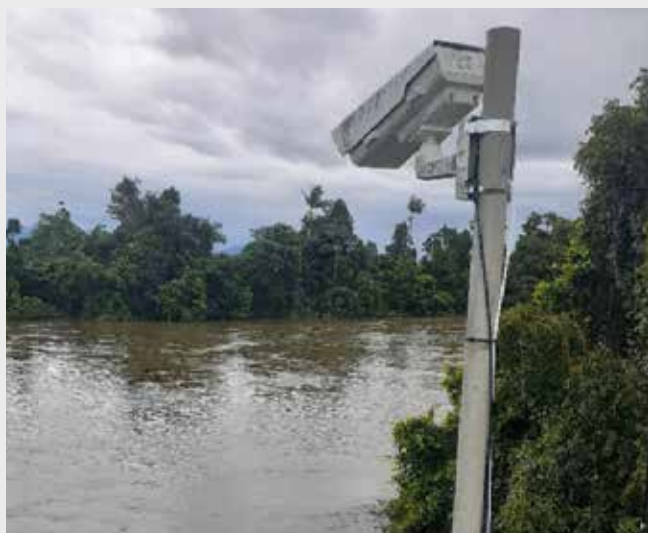
Figure 1. Fixed camera collecting videos for image velocimetry analysis.
