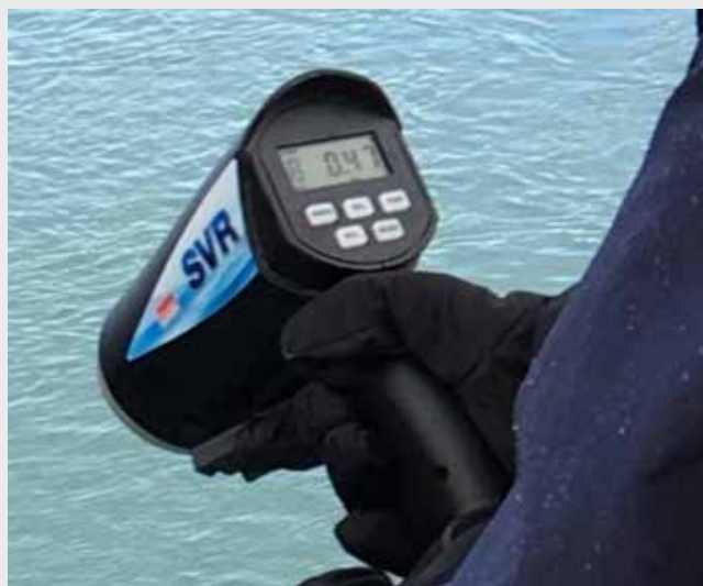
Figure 2. A handheld surface velocity radar gun (right). Source: Mark Randall.
