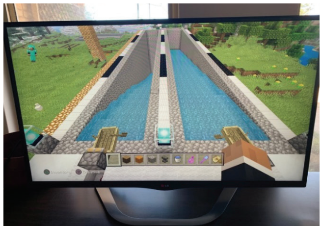
Figure 12. Use of boats in Minecraft to simulate a float gauging. Both boats are pushed into the channel simultaneously using redstone mechanism.
