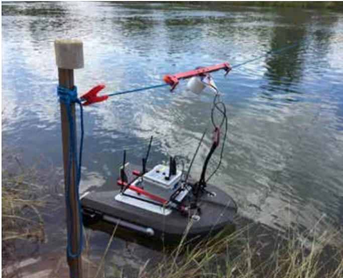
Figure 12. SonTek RS5 on ADCP Traveller – NIWA, M1 Channel.
