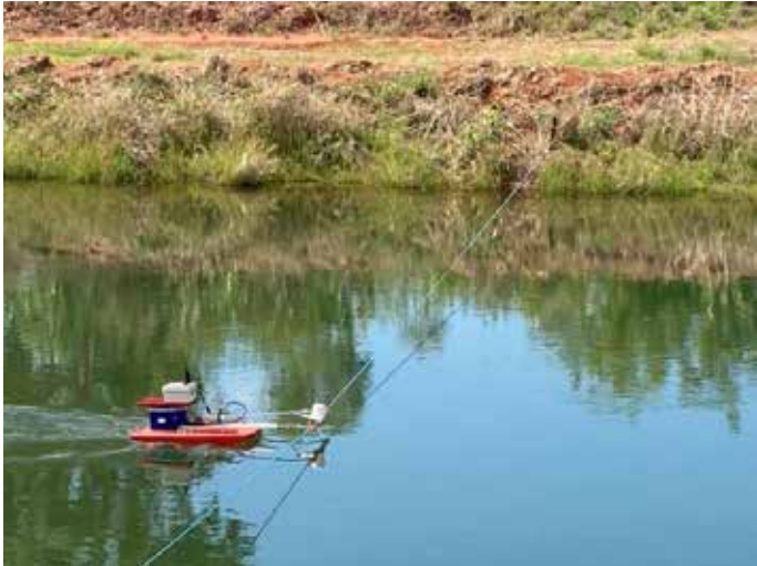
Figure 10. StreamPro ADCP Measurement.
