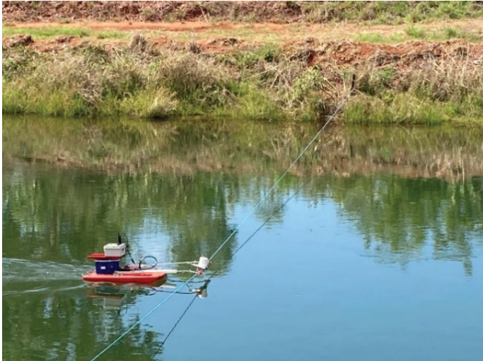
Figure 10. StreamPro ADCP Measurement.
