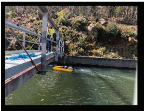
Images 3 & 4. Bronte Canal gauging bridge. Image 3 shows the winch/board arrangement for deploying the CM and columbus weight upstream of the bridge, and image 4 captures the ADCP secured slightly DS of the bridge.
