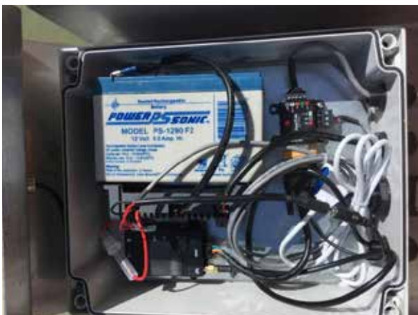
Figure 6. Junction box for housing electronics.
