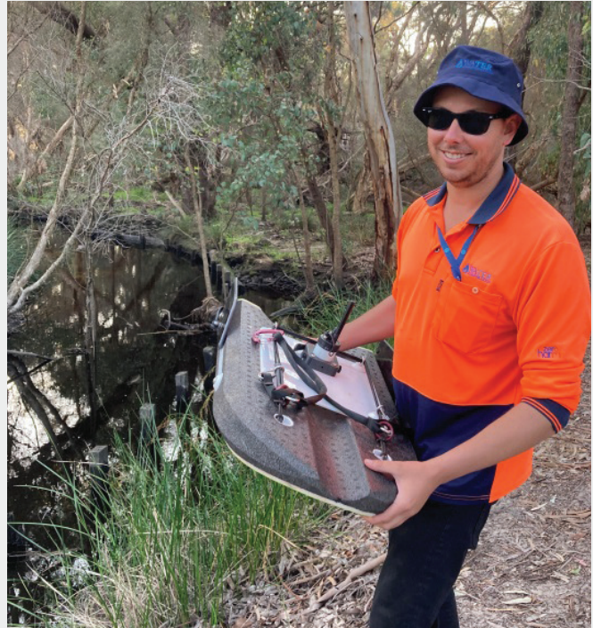
Figure 1. ADCP Measurement Bannister Ck.
