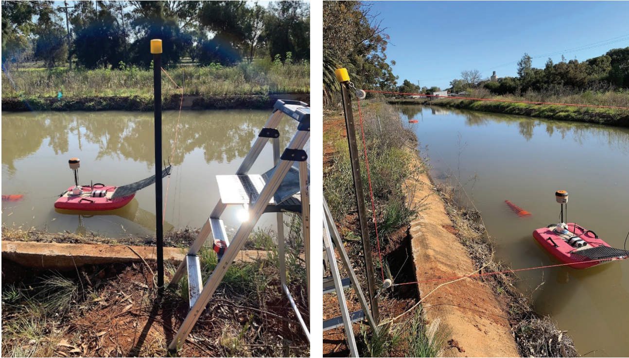
Figure 7. Cableway design at each measurement site for ADCP discharge measurements.
