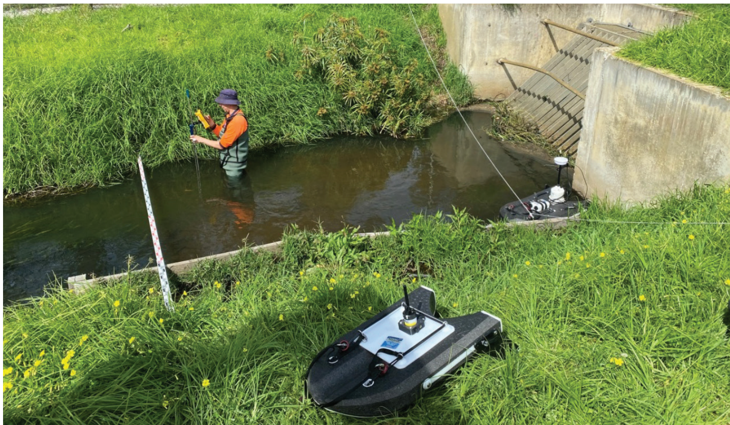
Figure 1. ADCP Measurement Bannister Ck.
