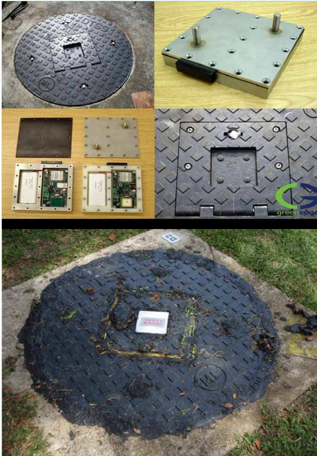
Figure 3. Manhole Opening Alarm System.
