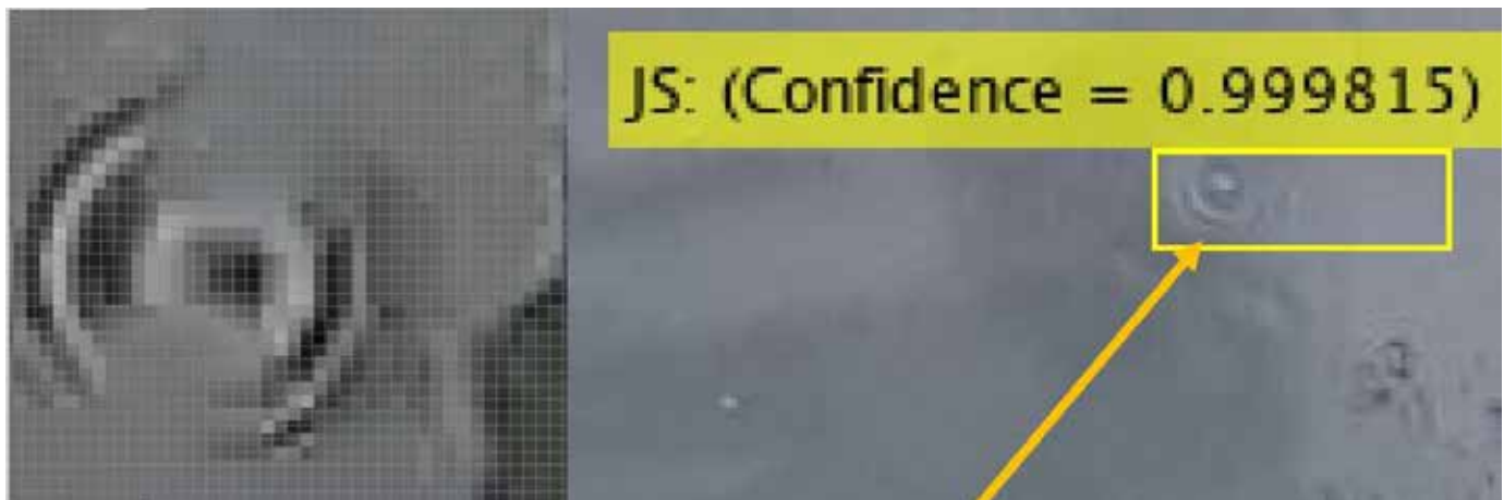
Figure 7: The Artificially Intelligent trained network detects a 'just-surfaced' bubble at the pixel limit of resolution.
