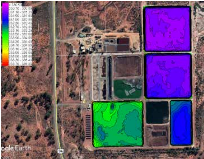
Figure 8: Sludge Surface Elevation.
