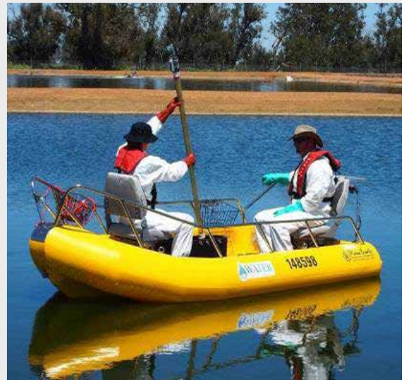
Figure 1: Water Corporation Hydrographers undertaking Sludge Profiling.
