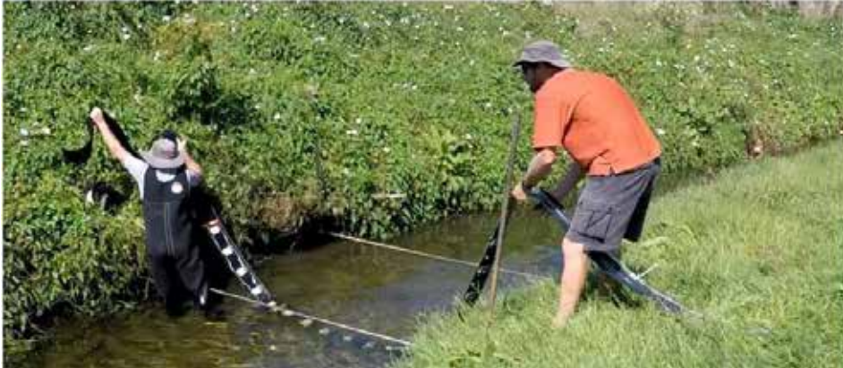
Figure 4: Left; Paul Hodgkinson and Thomas Wilding (HBRC) deploy the bubble line at Karewarewa Stream. Thomas did a lot of clearing and weeding on his previous visit to enable FlowTracker measurements. Right; snapshots of total discharge show good repeatability and agreement with the reference.
