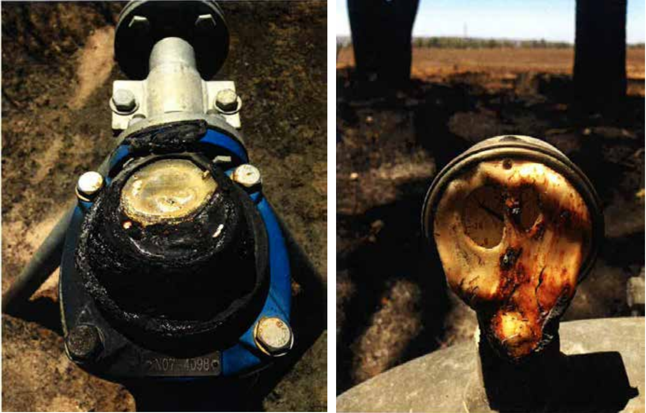
Figure 7: Example of Harvey Water Hydrometric Assets damaged by the Waroona Fire. Left: Mechanical Meter, Right: Pressure Gauge.
