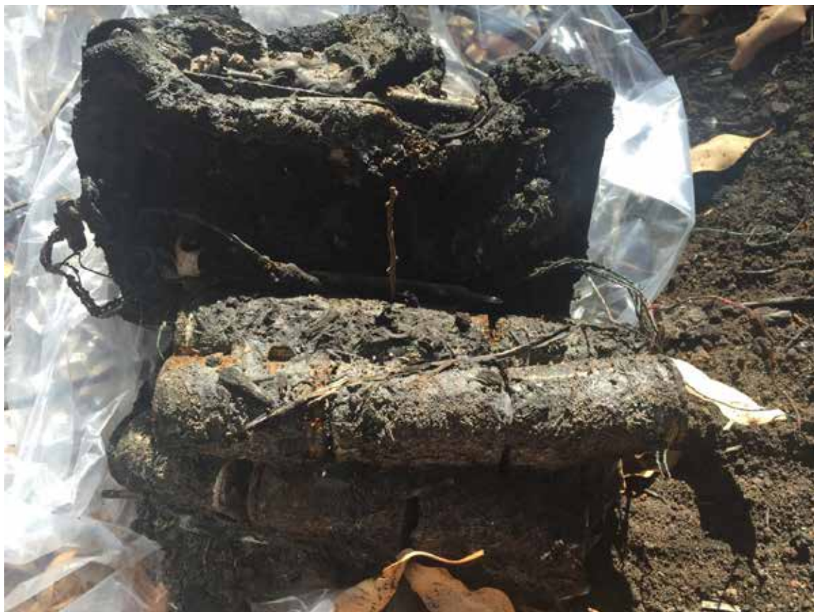
Figure 8: Damaged Logger from 6215W001 — Samson Brook at 1st Below Pipehead.
