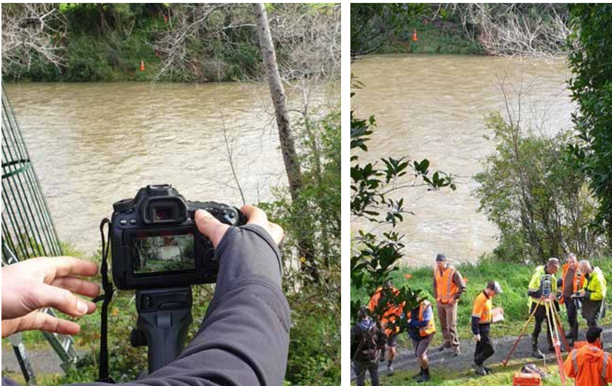
Figure 3: Left, “Fixed” camera installation setup. Right, Total Station survey of ground control points.
