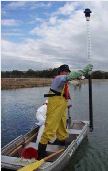
Figure 1: Water Corporation Hydrographers undertaking Sludge Profiling.
