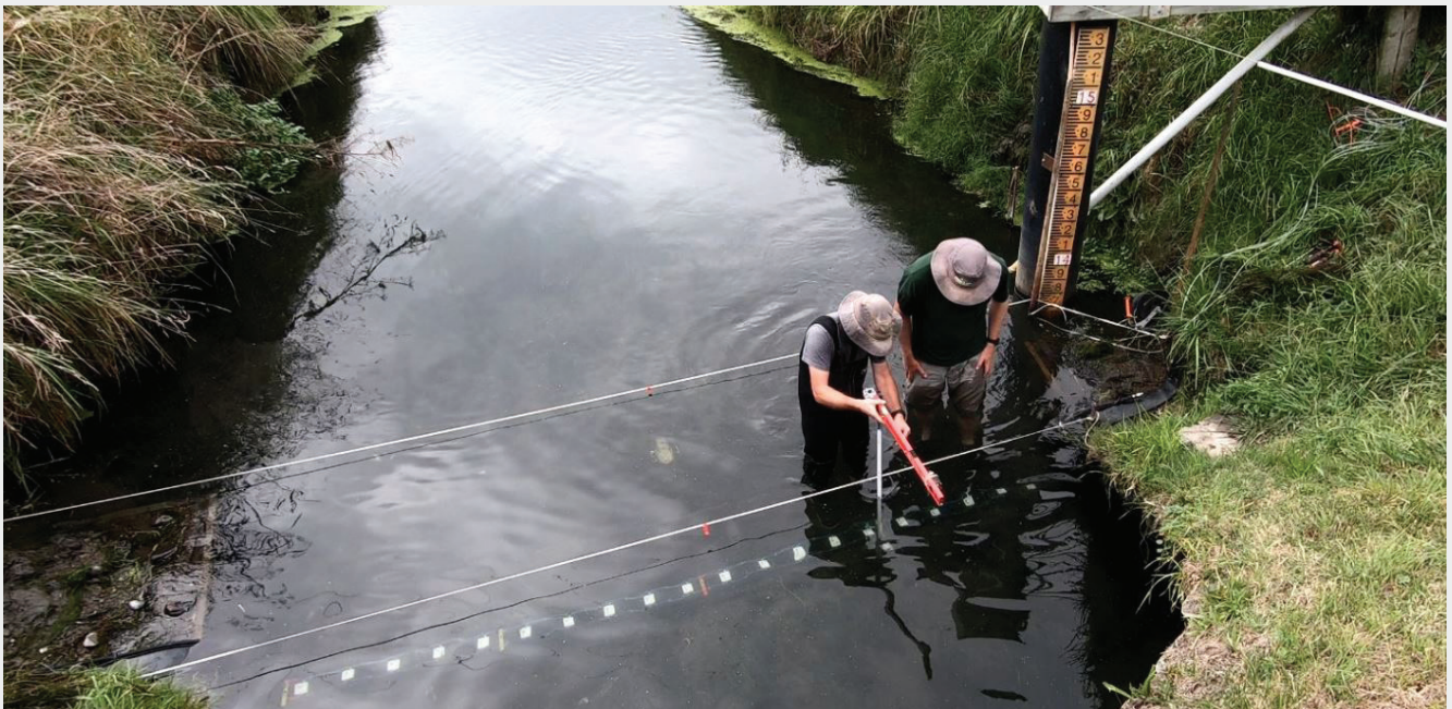
Figure 1: Paul Hodgkinson and Thomas Wilding (HBRC) deploy the bubble line within the Raupare Stream.
