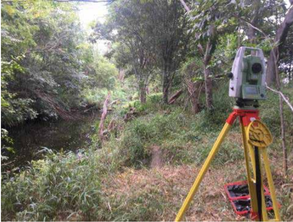
Figure 8: Leica Total Station.
