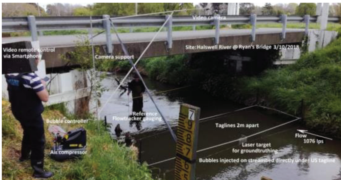
Figure 7: This is how we laid out the site for the trial on 3 October 2018. The water was flowing at over 1000 litres per second (L/s) and was quite turbid, so the bubble line is not visible.
