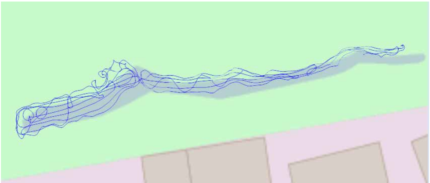
Figure 2: Q-Boat track during a stormwater pond survey, showing the coverage required to achieve a good bathymetric profile.
