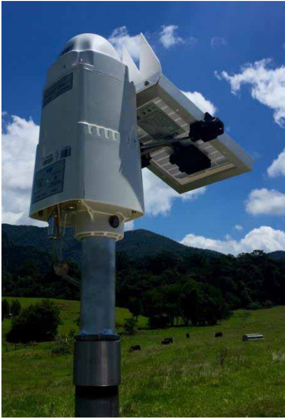
Figure 3. SatVUE pole mounted in the field.
