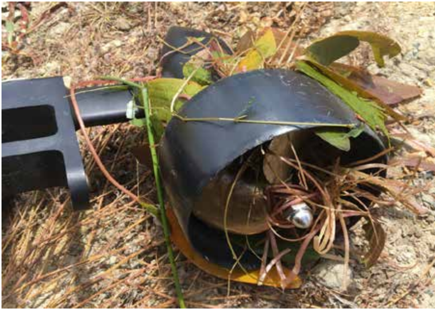
Figure 3: Q-Boat propeller clogged with weed.
