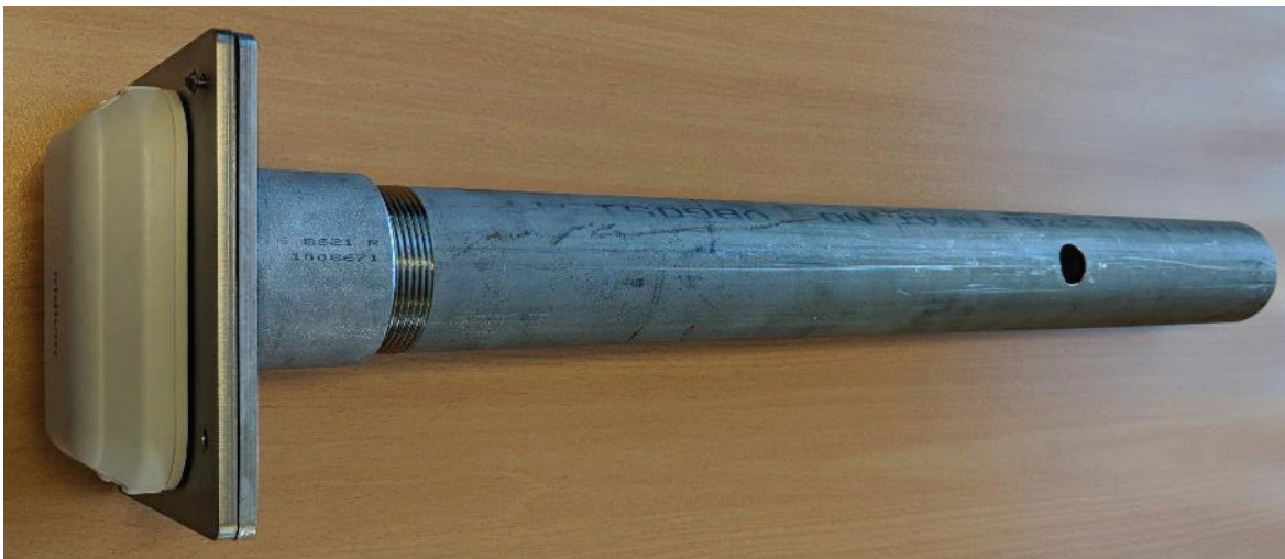
Figure 7. Iridium Edge module mounted on a 2" pole.
