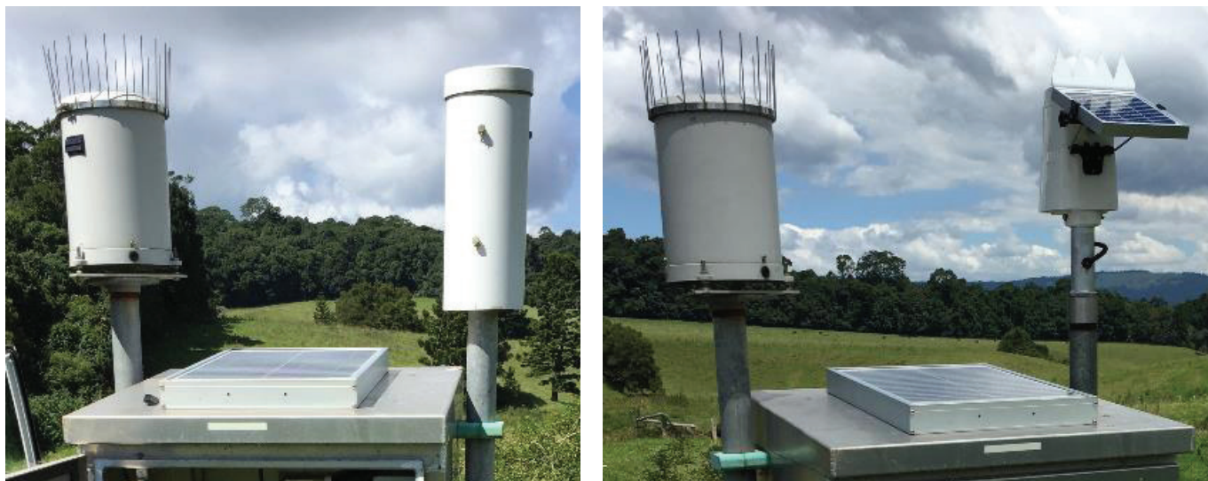
Figures 4 and 5. Before and after installation of SatVUE at Globalstar telemetry site.
