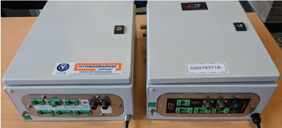
Figure 6. Old logger enclosure on the left, new XQ on the right.
