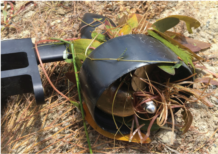
Figure 3: Q-Boat propeller clogged with weed.
