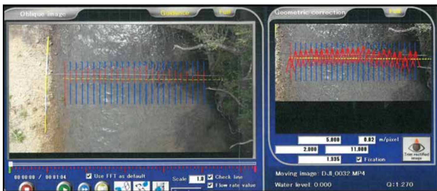
Figure 12. Low flow UAV measurements at Kolan River, Springfield. Ott C31 measured discharge 1.265 cumecs. Three separate UAV videos measured discharge as 1.213, 1.270, and 1.257 cumecs (data provided by Ray Maynard, DNRME, Bundaberg).
