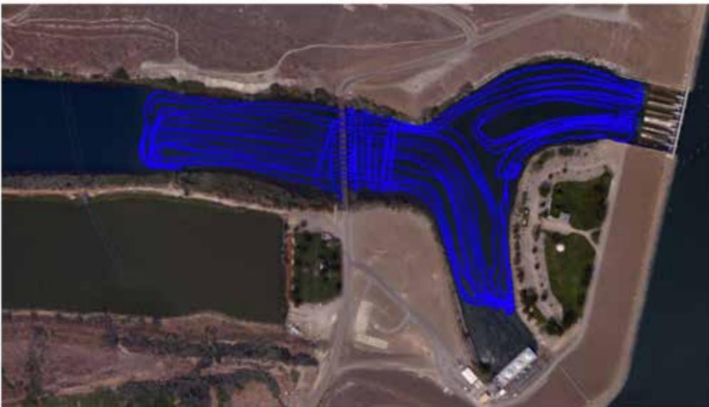
Figure 3. Survey Section on the Snake River below CJ Strike Dam showing ADCP survey track lines (courtesy of WaterCube, LLC).
