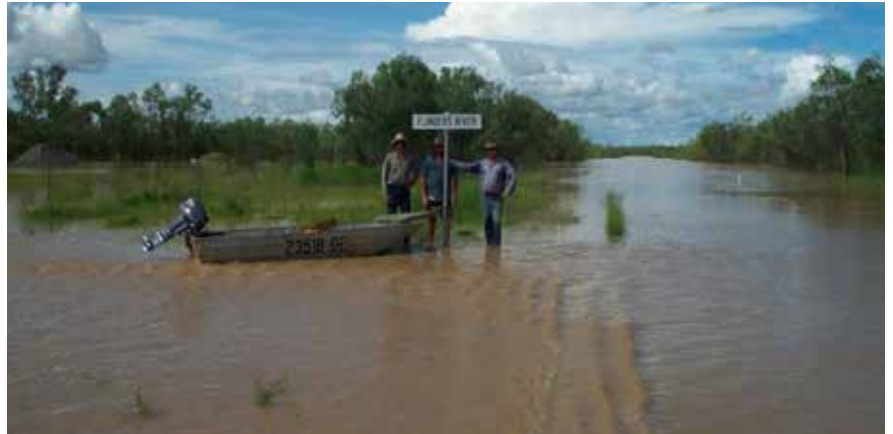
Figure 5. Remote area flood gauging at a section more than 2.6 km wide on the Flinders River at Walkers Bend (GH 12.00 m, Q 3618 cumecs).
