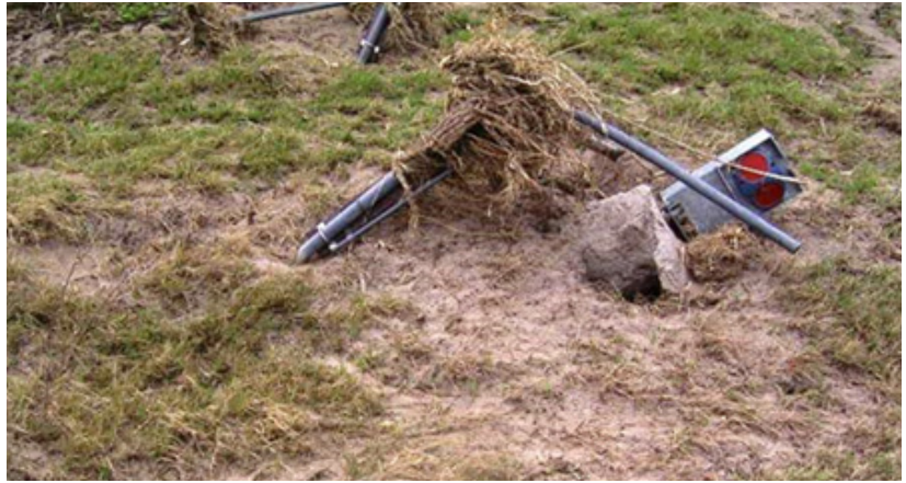
Figure 12. ADVM on Wide Bay Creek at Brooyar knocked over by a record flood GH 13.35 m in January 2013).
