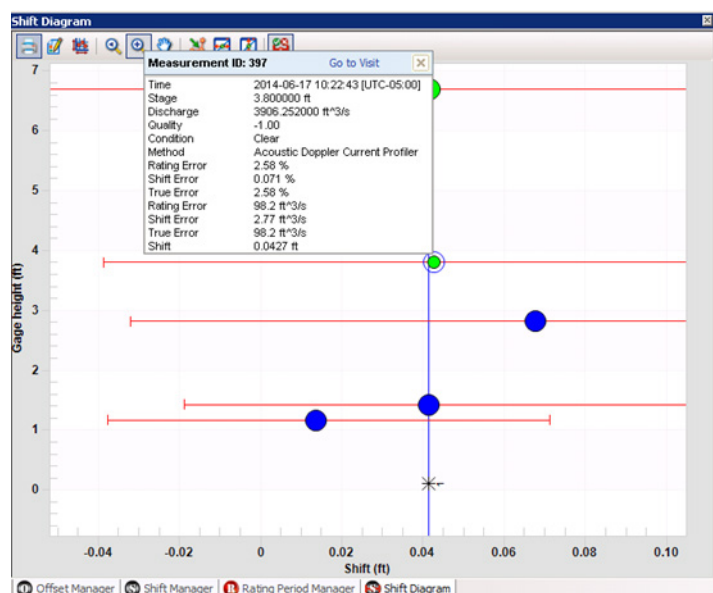
Figure 8a. Gauge Height versus Stage Deviation plot from USGS/WSC rating editor.
