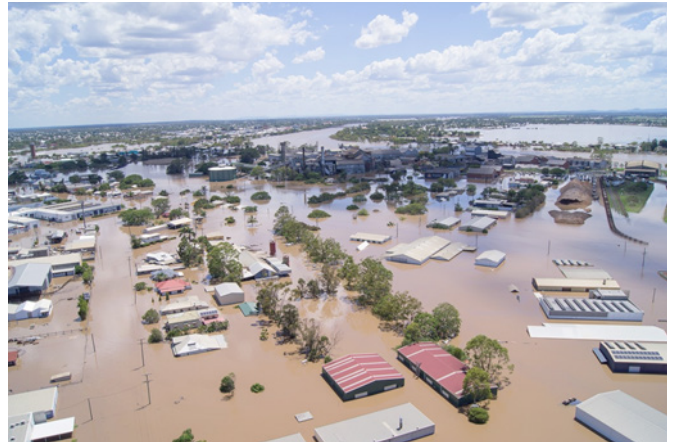
Figure 3. Burnett River January 2013 flood of almost 17000 cumecs in East Bundaberg (courtesy Rod Savidge).
