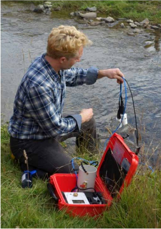
Gabe Sentlinger, Fathom Scientific, prepares sensors for salt dilution gauging at Mill Creek.
