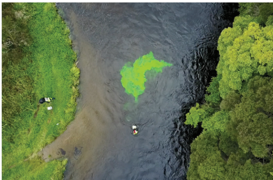
Flourescein tracer injection upstream of the regatta reach.
