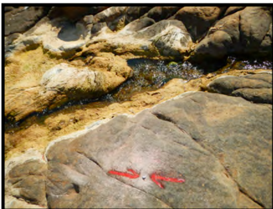
Figure 7: Control point on bedrock control.
