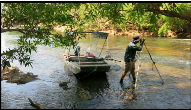
Figures 10 and 11: Surveying pool water levels into AHD using Dumpy Level.
