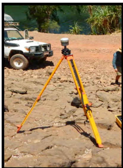
Figure 8: Static survey using Trimble R10.
