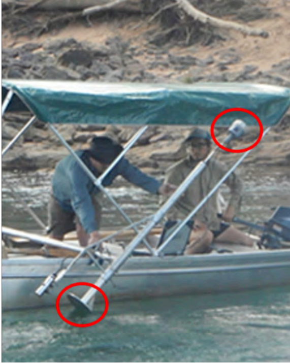
Figure 15: Trimble R10 GNSS Receiver and Tritech P/A500 Depth Sounder.
