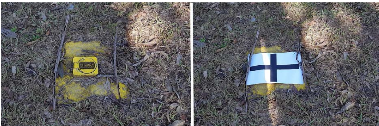
Figure 3: Primary Station benchmark (left). Ground Control Point target (right).
