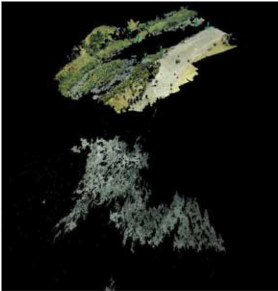
Figure 4: Pre-processing of point cloud showing terrain model with superfluous data interpolated by cloud reflections on water surface.
