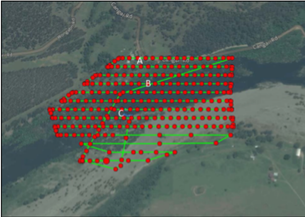
Figure 2: UAV transect of Jackadgery site showing Station (A), Sensor (B) and Control (C).
