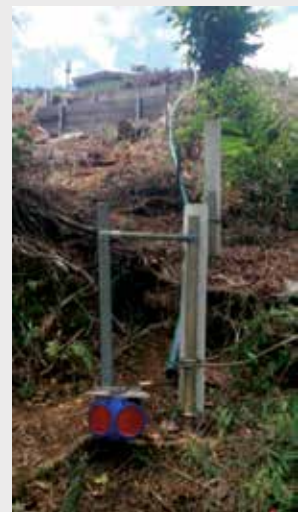
HADCP setup on gauge line.
