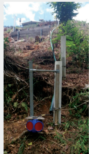
HADCP setup on gauge line.
