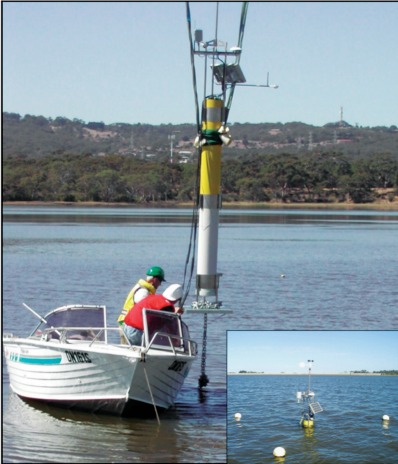
Figure 9. A MEA spar-buoy supporting three separate thermistor strings having different anchoring arrangements to allow stratification monitoring in the epilimnion (surface layer), metalimnion (thermocline layer) and hypolimnion (bottom layer) of a reservoir, no matter how the water level changes. The perforated plate at the bottom of the buoy acts as a hydraulic damper to prevent the buoy 'bobbing' in rough water. The length of the chain wrapped around this damper plate is adjusted to change the flotation depth of the spar buoy, which sits low in the water (bottom, right) to allow correct operation of the net radiometer. The latter is part of the weather station cluster mounted on the buoy to monitor wind and solar energy. The station uses cellular phone long-haul telemetry and VHF ship-to-shore SCADA radio systems.
