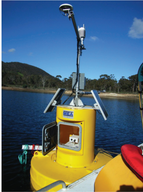
Figure 8. This Sealite buoy supports a full MEA logging system, an integrated weather station capsule (Vaisala WXT-510) for air temperature, relative humidity, (drum-head) rainfall sensor, barometric pressure, ultrasonic wind speed and direction and separate global solar and net radiation sensors. All of these sensors are SDI-12 compatible, as is the MEA electronic compass (seen through the instrument door) developed to give a local reference direction for the wind direction sensor. The data logger reads only SDI-12 sensors, and includes Next-G cellular-phone telemetry for remote data collection.
