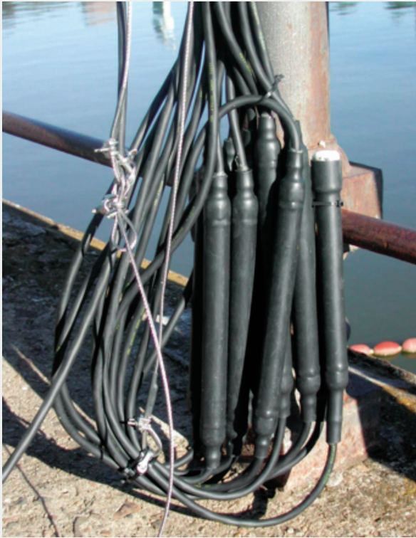
Figure 2. An MEA temperature sensor string bundled together for two-point in-field calibration at the Torrens Lake in Adelaide South Australia. Lots of effort went into keeping water out. Sensors are large so that their thermal mass acts to filter out turbulence-induced temperature variations at a five minute logging rate.
