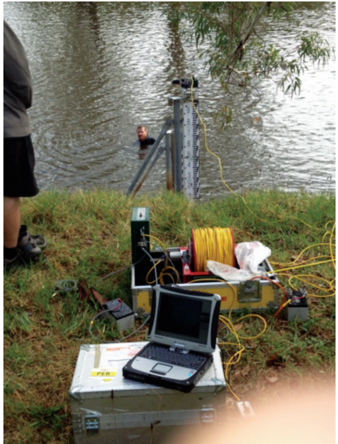
Bore hole camera being fed into inlet.
