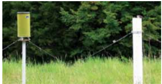
Automatic rain gauge and storage gauge at Third House.
