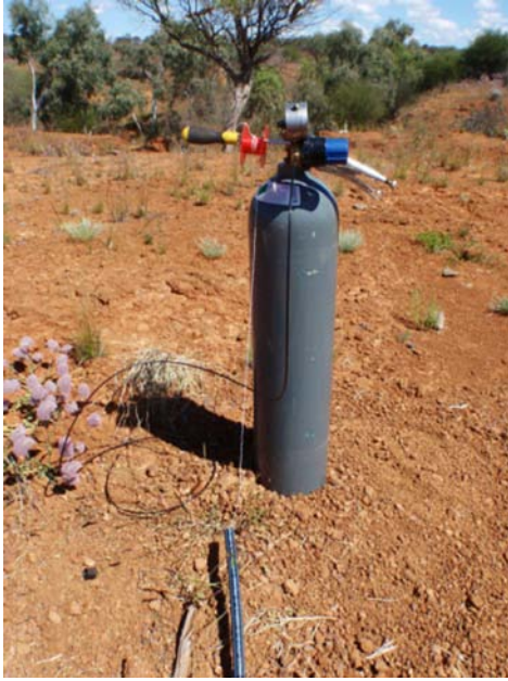
String feed nitrogen propulsion system.
