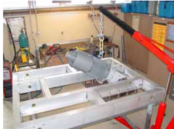
Installing the drive line
