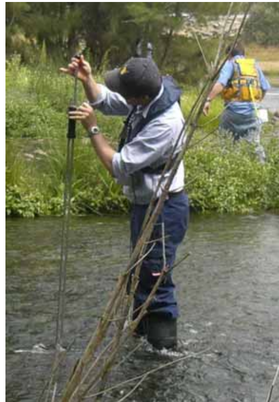
Undertaking current meter gauging experience.
