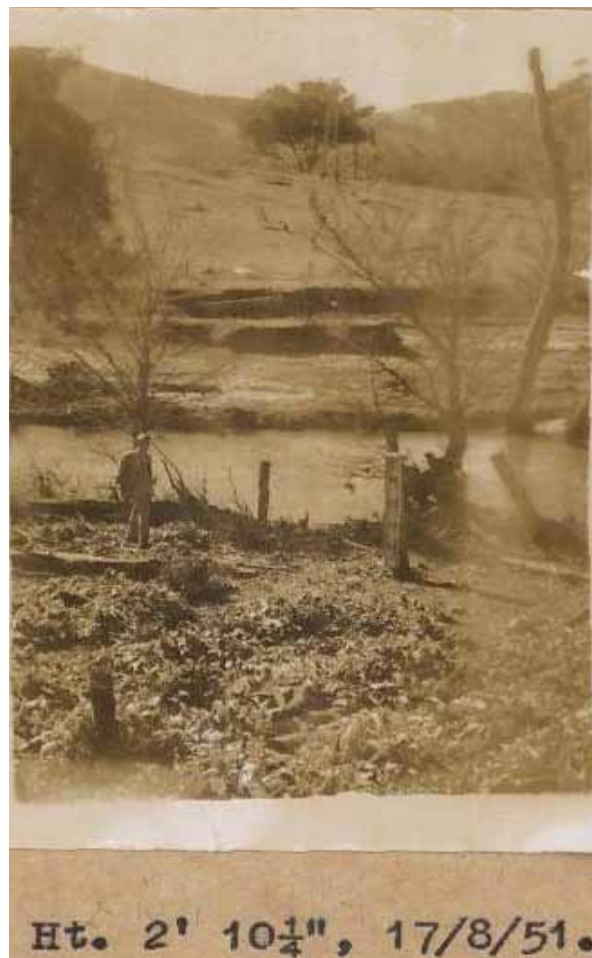
Photograph . Adjungbilly Creek at Darbalara (410038) gauging station with staff gauges. Gauge readers house approximately 50 distant.
