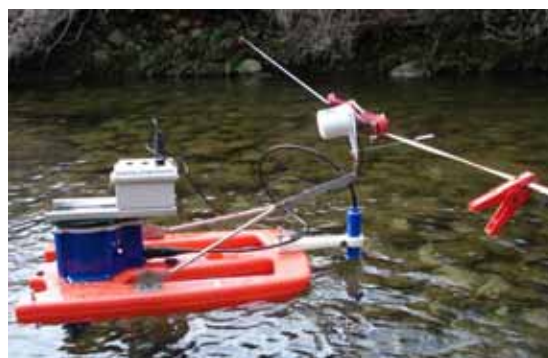
Figure 2: Traveller attached directly to the StreamPro towing bridle.
