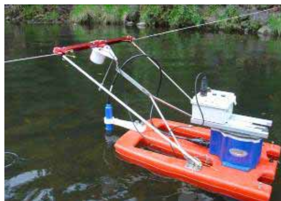
Figure 3: Traveller connected to the StreamPro at 3 points to minimise float swimming motion.
