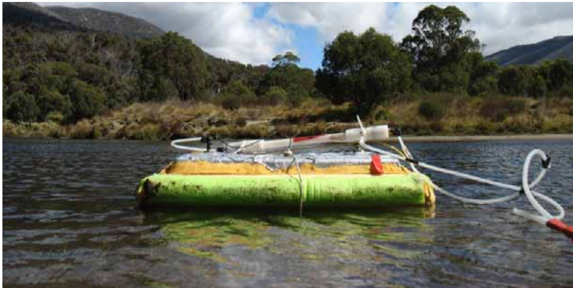
A low down view of the measuring chamber that floats on the water surface collecting the methane fluxes
