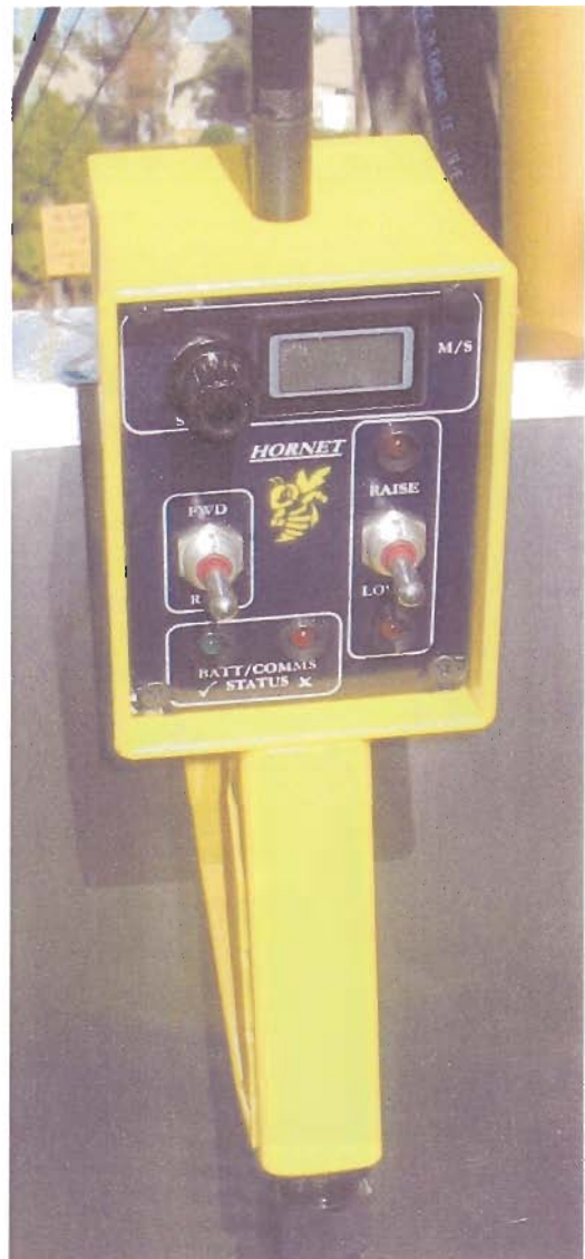
The simple to use control pad with variable traversing speed facility and traverse speed indicator
