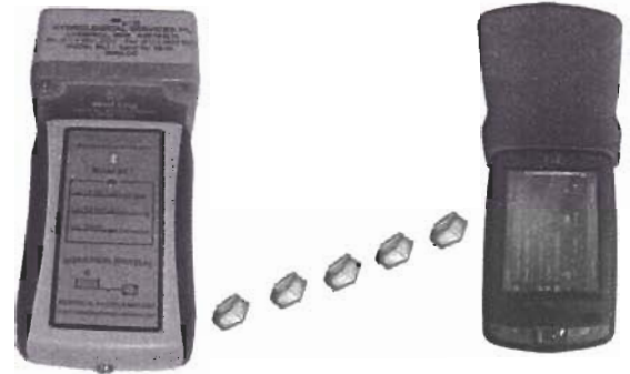
Figure1. BlueComms Connected to a Minilog, Communicating to a PDA Using Wireless Bluetooth™ Technology.
