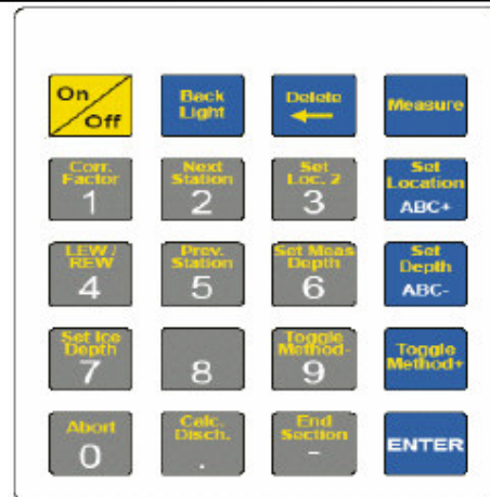
2.2a FlowTracker handheld controller keypad
