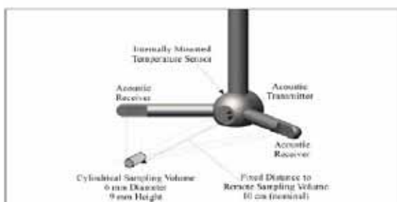
2.3b The FlowTracker probe detail.
