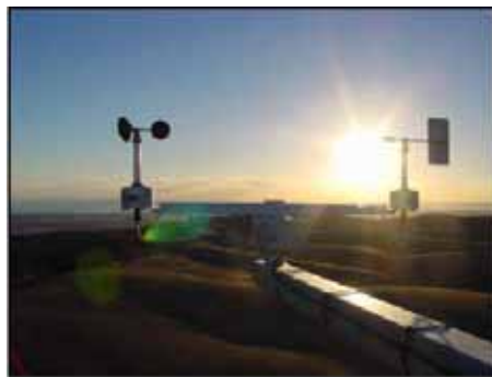
Figure 3.2 Anemometer and Vane from top of 70m mast in SA.
