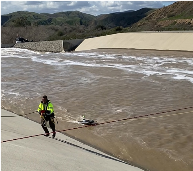
Figure 4: ADCP Streamflow gaugings with RiverSurveyor M9 and RS5. High flow conditions left, low flow conditions right.
