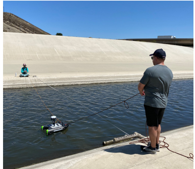
Figure 4: ADCP Streamflow gaugings with RiverSurveyor M9 and RS5. High flow conditions left, low flow conditions right.
