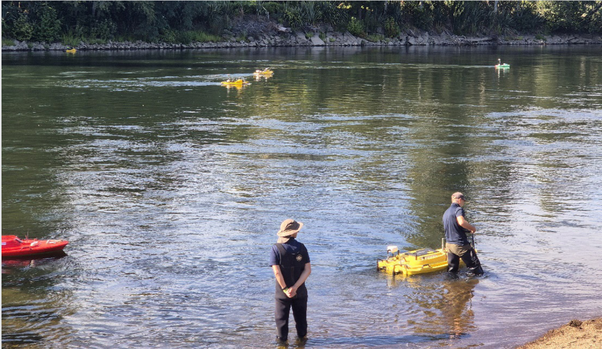
Figure 4: Surfbees, Arcboats, QBoats and RQPod in use during the Flow Measurement Regatta
