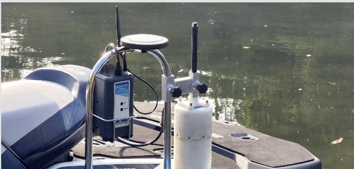
Figure 3: Close up of ADCP mounted on the Waikato Harbourmaster vessel
