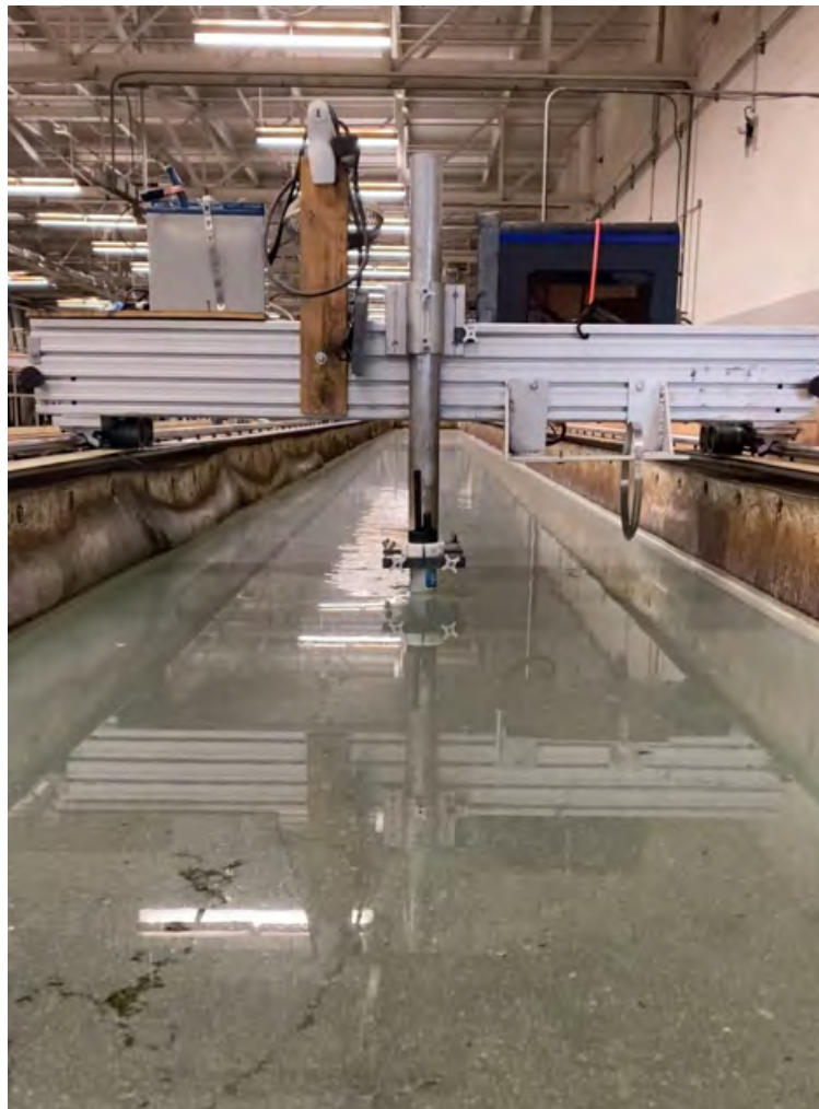
Figure 2. "SonTek RS5" in the Process of being Verified following "USGS" Process at the HIF.
