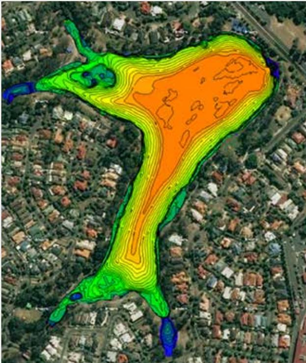
A Survey was performed of a residential lake to determine the total volume of sediment deposited. The survey comprised of the main water body and four inlets discharging into the lake. The survey methods applied during the bathymetry survey varied from bathymetric survey using unmanned surface vehicle/dual frequency echo sounder to topographic survey of the banks and inlets using survey rod and data collector.
