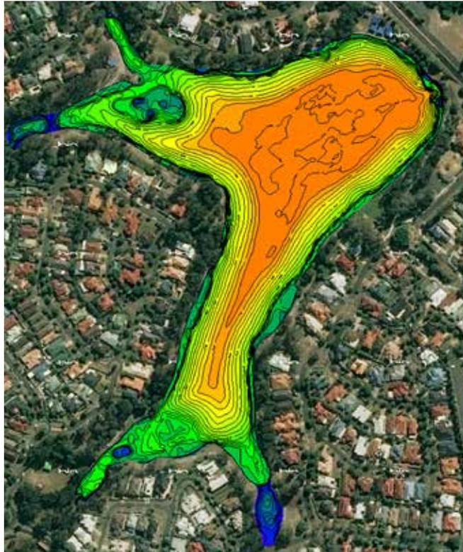
Figure 16. Channel Bed Surface Elevation.
