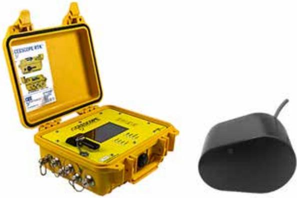
Figure 2. CEESCOPE & M195 Dual Frequency Echo sounder.
